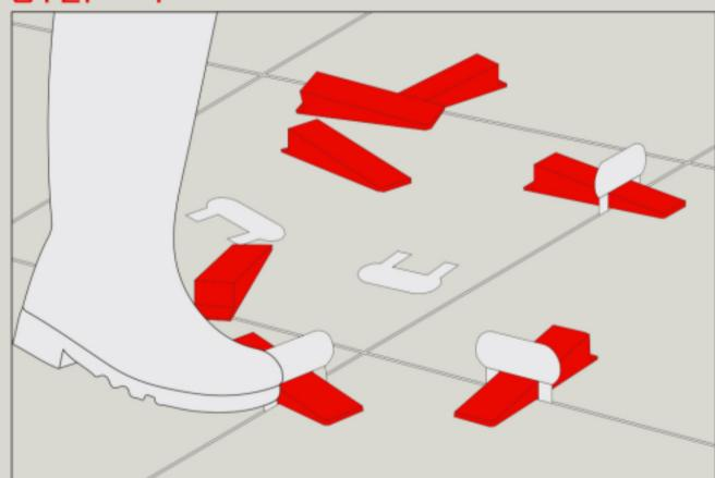
AFTER ADHESIVE DRIES, BREAK OF LOOSE ENDS WITH RUBBER HAMMER OR KICK OFF WITH BOOT.
