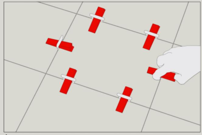
INSERT WEDGE INTO CLIP, PLACE THUMB ON BACK SIDE OF WEDGE AND PLACE MIDDLE AND FOREFINGERS ON CLIP.
