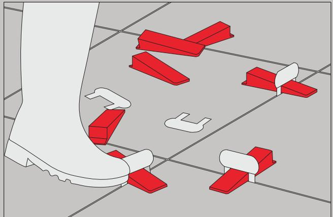
NACH DEM DER KLEBSTOFF GETROCKNET IST, BRECHEN SIE DIE LOSEN ENDE MIT EINEM GUMMIHAMMER ODER MIT EINEM KICK MIT IHRER STIEFEL. AFTER ADHESIVE DRIES, BREAK OF LOOSE ENDS WITH RUBBER HAMMER OR KICK OFF WITH BOOT.
